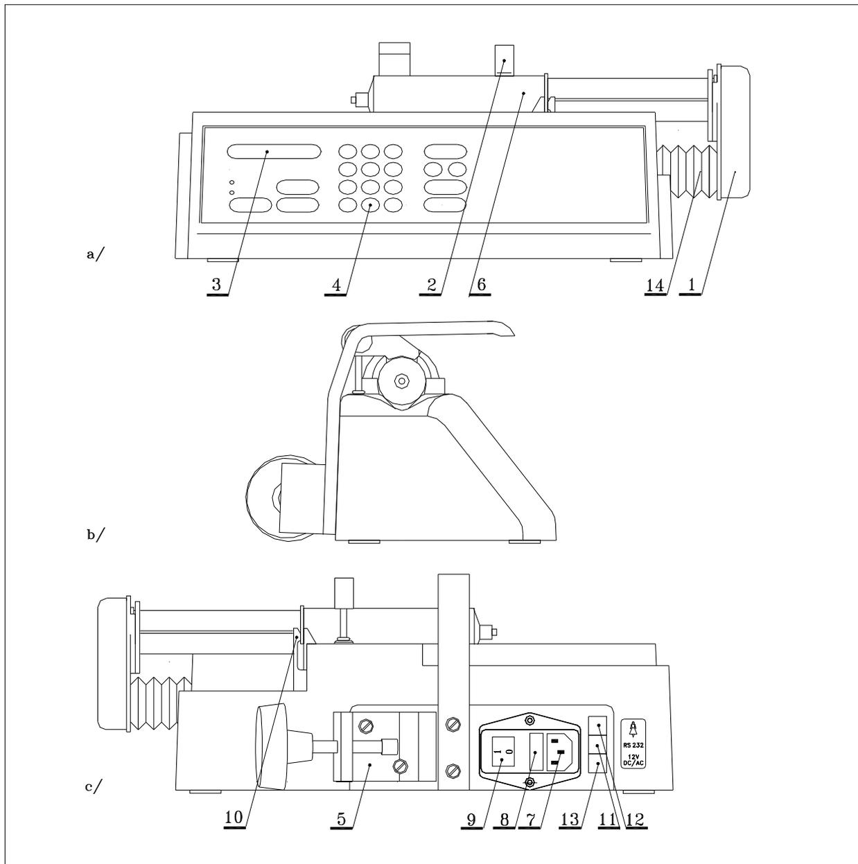
Fig. 1. **Pump AP 12, view from:** a) front , b) side , c) back
