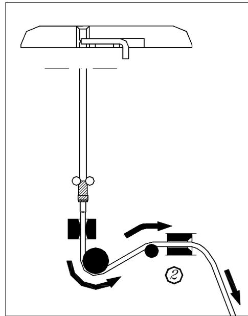
2. Install the infusion set accordingly to the drawing – it should go through the air bubble sensor, then lay along the round guide pins and go outside the pump.
