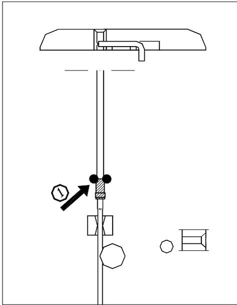
1. Installation of the infusion set should begin from the bottom part of the silicone insertion. Insert it under the round holders.
