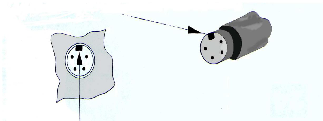
3. Softly slip the plug in until resistance is felt.
