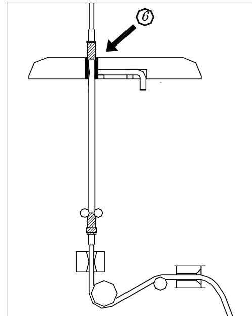
6. Close the pump door. Thanks to its elasticity, the infusion set will shrink and take the proper place
